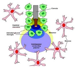
Conductive polymers can improve interactions between metallic electrode and living cells with high ionic/electronic conductivity in bioelectronics. Melanin has been studied as a natural material with non-toxicity, high adhesion to inorganic surfaces, and stability in aqueous environments.
